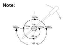
When using the hand lever to apply pressure to the jaws, ensure the closing force is a minimum of twice the weight of the load being hoisted.
