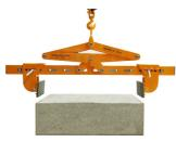
**Step 3:** Adjust the gripping range of the lifter so that it is suitable for size of block to pick up.
