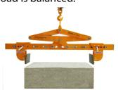
**Step 6:** Raise the hoist to allow clamping jaws to close onto the load. Then lift and move the block slowly so that the load is balanced to desired location.
