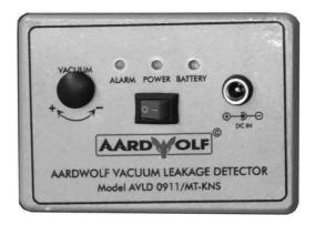
Aardwolf Vacuum Leakage Detector is a battery powered unit consisting of a pressure sensor, an audible warning red warning light and test switch, all controlled by a solid state microchip. It is equipped with a rechargeable Lipo 1-cell battery with a capacity of 3.7V - 2000mAh and the working mode up to 20 operating hours.
