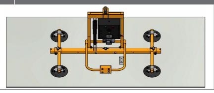
STEP 6 | Manually adjust the cross bar and stringer beam based on the shit size
