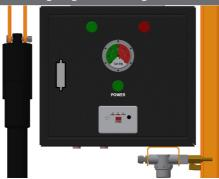
**Caution:** In that case, nidle on the vacuum gauge is not reaching 53 kPa (40 CmHg) and it is still in the red zone, the red vacuum light is on, the alarm warning system rings, this means that the vacuum is not full and the lifter cannot lift the load
