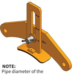
**Third:** Screw the bolt back and make sure that it is tight before lifting.
