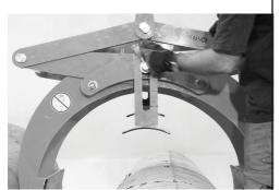
**Second:** Move the top pad to the required diameter position.
