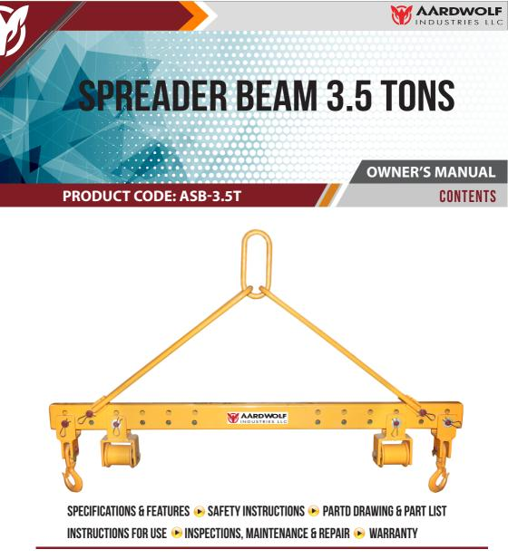
Specifically designed for the stone industry. The Spreader Beam, in combination with endless slings, is an invaluable piece of equipment where stone is required to be rolled over. The slings are suspended on crowned aluminium rollers. This makes turning the load in the sling easier. The rollers will handle up to 90mm wide slings. The swivel hooks can be used in place of rollers. The overall width is 2000mm.
