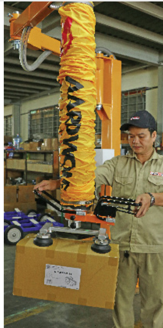
The lifting tube is covered by protective fabric.
