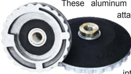
These aluminum backer plates are attached to the polishing tool and each of the pads has a snail lock adapter. The adapter simply fits into place and locks on with a twisting motion. To remove the pads simply untwist and remove, then replace it with the next grit.
